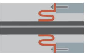
5. **Collar** of the compensating wall penetration seal has to be **adjusted** untill a **stretching mark** appears. **Inject sealant** under collar circularly and **warp strap closely**.
