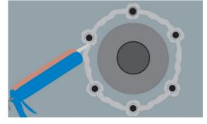
Pull open side (at the flange side) of the compensating wall penetration seal type VDW over the casing pipe. Warp compensating wall penetration seal type VDW with pressure plate against the wall / ceiling. Spread oozed sealant.
