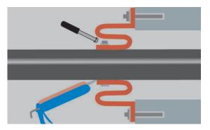
For **laying underground** the **compensating wall penetration seal has to be covered with a stretching cusion** before filling to prevent compensating wall penetration seal of earth burden. This **allows the movement of the compensating wall penetration seal**.
